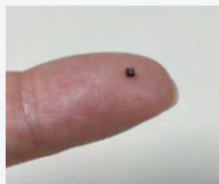
Amtelus®, the world's smallest light emitting device
