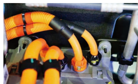
High-voltage cables used in electric vehicles
