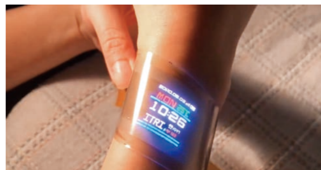
Flexible mini-LED display using materials from Shin-Etsu Chemical
