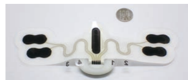
Health patch using Shin-Etsu Chemical's materials for wearable devices. The black-colored parts are the electrophysiological dry electrodes and the gold-colored lines connecting them are the high-stretchable wiring.
