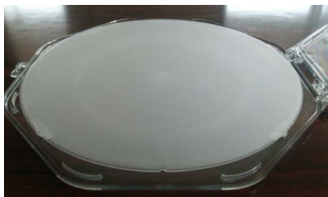
Figure 1 Image of Shin-Etsu's single-side-polished synthetic quartz wafer
