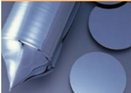
Single crystal silicon ingot and wafers
