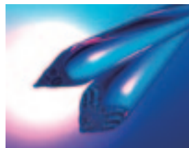
Optical fiber preform with diameters of 200mm and lengths of 2,000m
