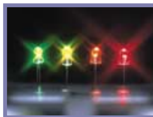
Epoxy molding compounds, which are silicone variations, are necessary materials for high-intensity LEDs.
