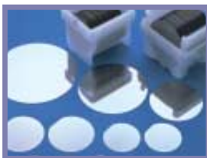
Silicon wafers boast a degree of evenness to within 100 nanometers.
