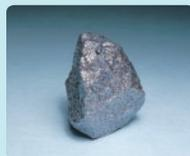
Silicon metal is produced by the endothermic reduction of quartz. This is a key raw material in the production of silicone, semiconductor silicon, synthetic quartz, solar cells and many other products.
