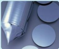
Silicon wafers are used as substrates of semiconductor devices, which are vital to electronics such as PCs, smartphones, digital home appliances and automotive devices. Technological requirements on these wafers have
