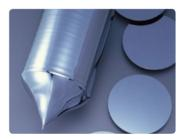
Single crystal silicon ingot and wafers
