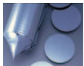
Single crystal silicon ingot and wafers
