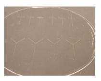
\* (Example) The above Micro channel: width x depth=50×20um
