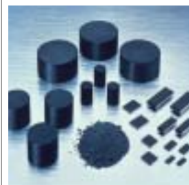
Epoxy molding compounds prevent semiconductor circuit leaks, protect regular and large-scale circuits from humidity, and are outstanding in terms of heat and shock-resistance.
