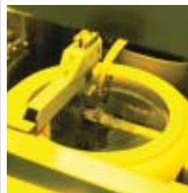
Photoresist spin-coated onto a wafer
