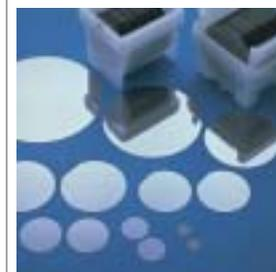
Silicon wafers boast a degree of evenness to within 0.1 micrometer.
