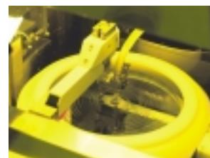
Photoresist spin-coated onto a wafer
