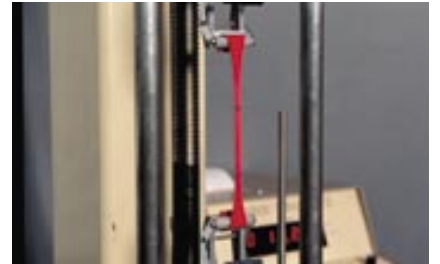
Testing the tensile strength of Silicone Rubber
