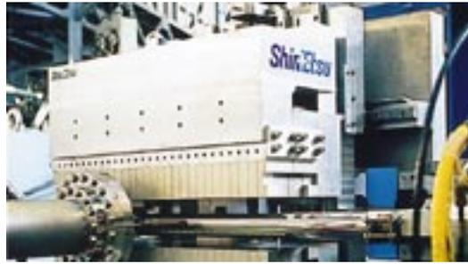
*Variable polarizing undulators, in which rare earth magnets are a critical component, are used as the light source for synchrotron radiation.*
