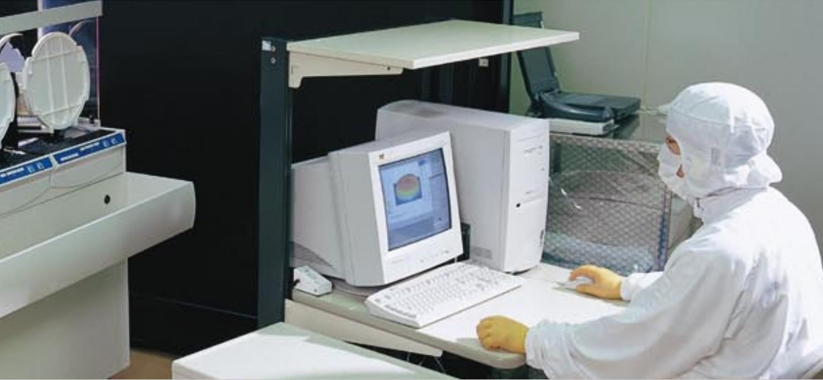
*The production of 300mm-diameter silicon wafers demands the highest level of technology at every step through final testing. Shown here is the critical surface finish inspection.*
