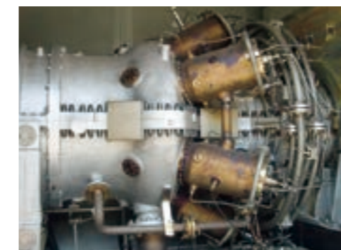
Power generation gas turbine
