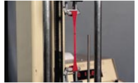
Testing the tensile strength of Silicone Rubber
