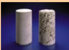
Concrete samples with (left) and without (right) Usca Clean additive
